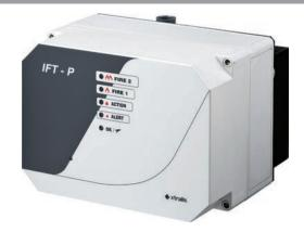
The ICAM IFT-P detector is an air-sampling system with an alarm sensitivity range from 0.0003% to 6.10% obscuration/ft (0.001% to 20% obscuration/m). This detector is classified as a Very Early Warning Smoke Detector that can reliably detect fire at an early stage, and low to high concentrations of smoke over an area of up to 21,500 ft² (2000 m²).
