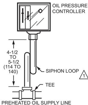
⚠ 1/4 INCH PIPE WITH 1/4-18 NPT EXTERNAL THREADS ON BOTH ENDS AND 2-1/4 IN. (57 MM) DIAMETER LOOP.
