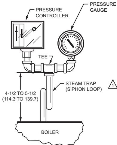
1 1/4 IN. PIPE WITH 1/4 - 18 NPT EXTERNAL THREADS ON BOTH ENDS AND 2-1/4 IN. DIAMETER LOOP.
