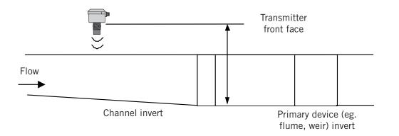
In addition to the above, when setting the bottom reference on a 'V' notch weir it is important that the true invert of the weir is taken and not the meniscus liquid level, which may be 3 to 4mm (1/8") above the true invert.
