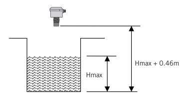
It is important to note that the bottom reference of the transmitter should be related to the centre of the invert of the primary device, NOT the distance to the channel bottom directly below the transmitter.
