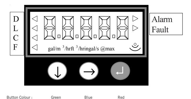
The main display allows display of up to 5 characters, which in the normal run mode will be the measurement, termed the Primary Variable (PV) of the instrument, or in the programming mode will be data to assist in programming.
