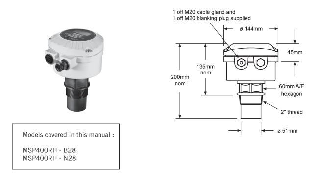
The transmitter is mounted using the 2" thread provided. An optional mounting bracket kit is available on request. MSP-BRK2 (2" BSPT) or MSP-BRK3 (2" NPT).
