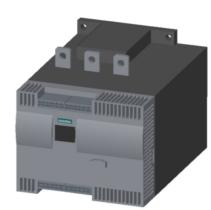
SIRIUS soft starter Values at 400 V, 40 °C standard: 432 A, 250 kW Inside-delta: 748 A, 400 kW 200-460 V AC, 230 V AC spring-type terminals !!! Phased-out product !!! Successor is SIRIUS 3RW5, Preferred successor type is >>3RW5547-2HA14<<
