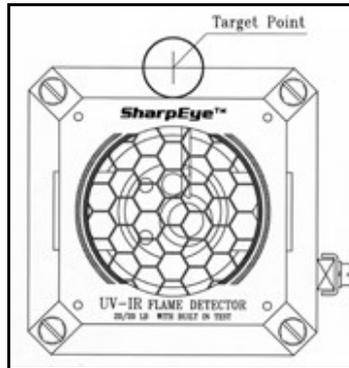
*Figure 14: UV/IR Detector Target Point*
