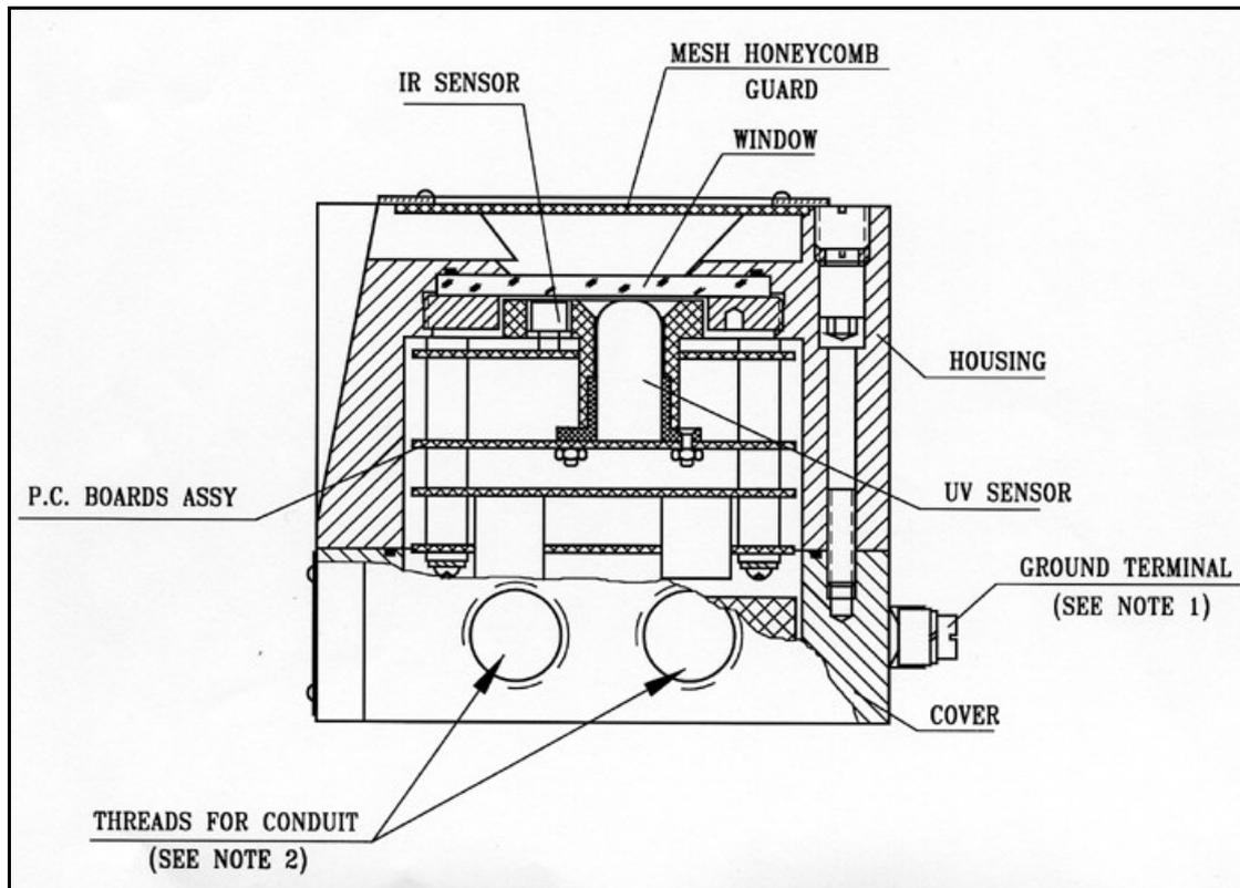
*Figure 2. Flame Detector Assembly - Schematic Section*
