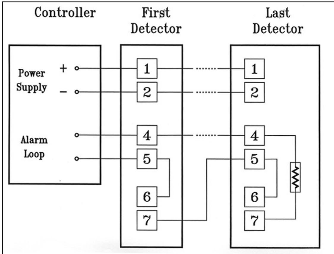
Figure 8. Typical Wiring Diagram for Four-Wire Controller
