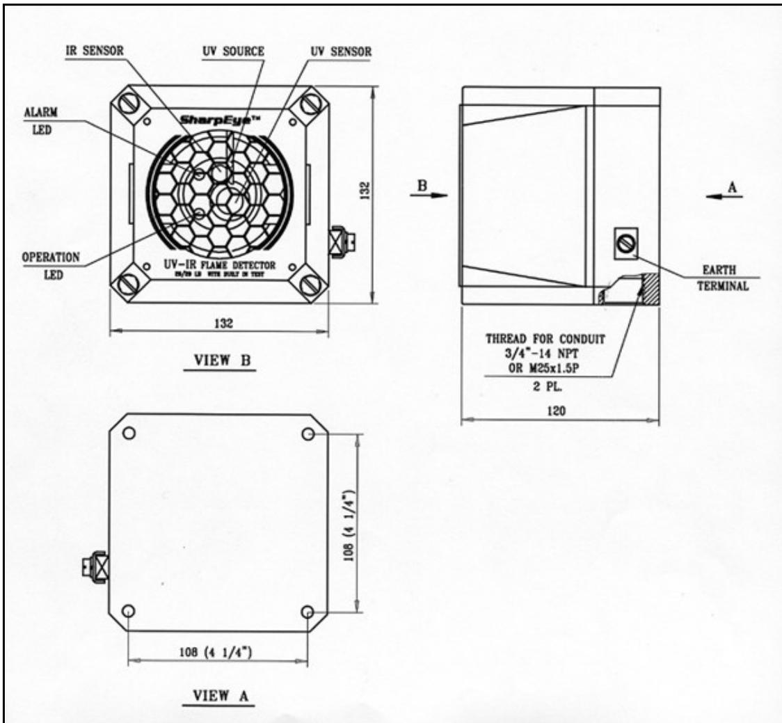
Figure 1. Flame Detector Assembly - Outline Drawing
