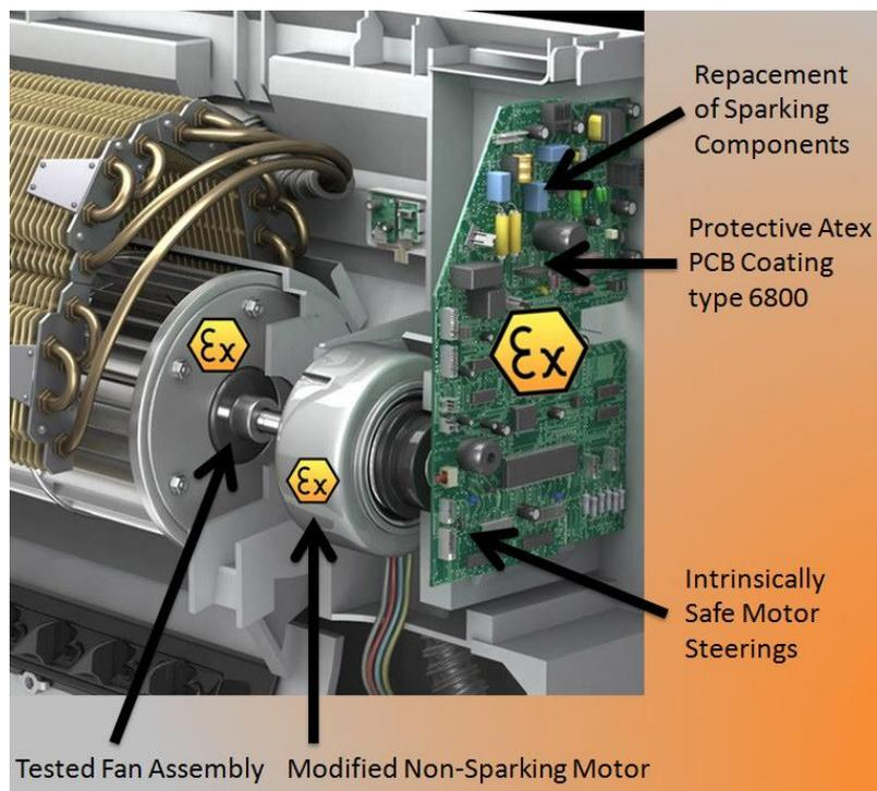
The above picture demonstrates some of the protective anti-explosion measures intergraded in Atexxo's indoor unit. All modifications are according to safety standards, well documented and tested. Standard units are available from Daikin, other brands can be delivered on request.
