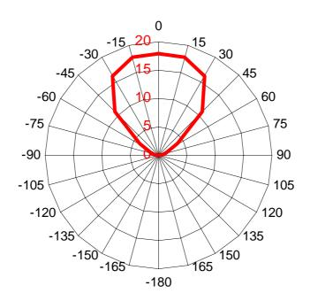
The detectors have a horizontal field of view of 90 degrees, with the greatest sensitivity lying along the central axis. This is indicated in diagram 1 which shows field of view in degrees plotted against distance in metres.
